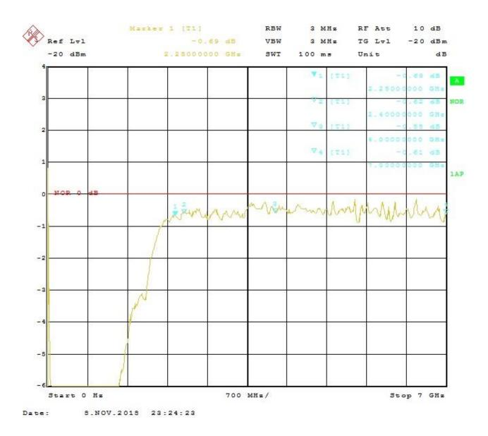
The insertion loss in the range ~2 GHz to 7 GHz is below 1dB. Here are some measurement points:
