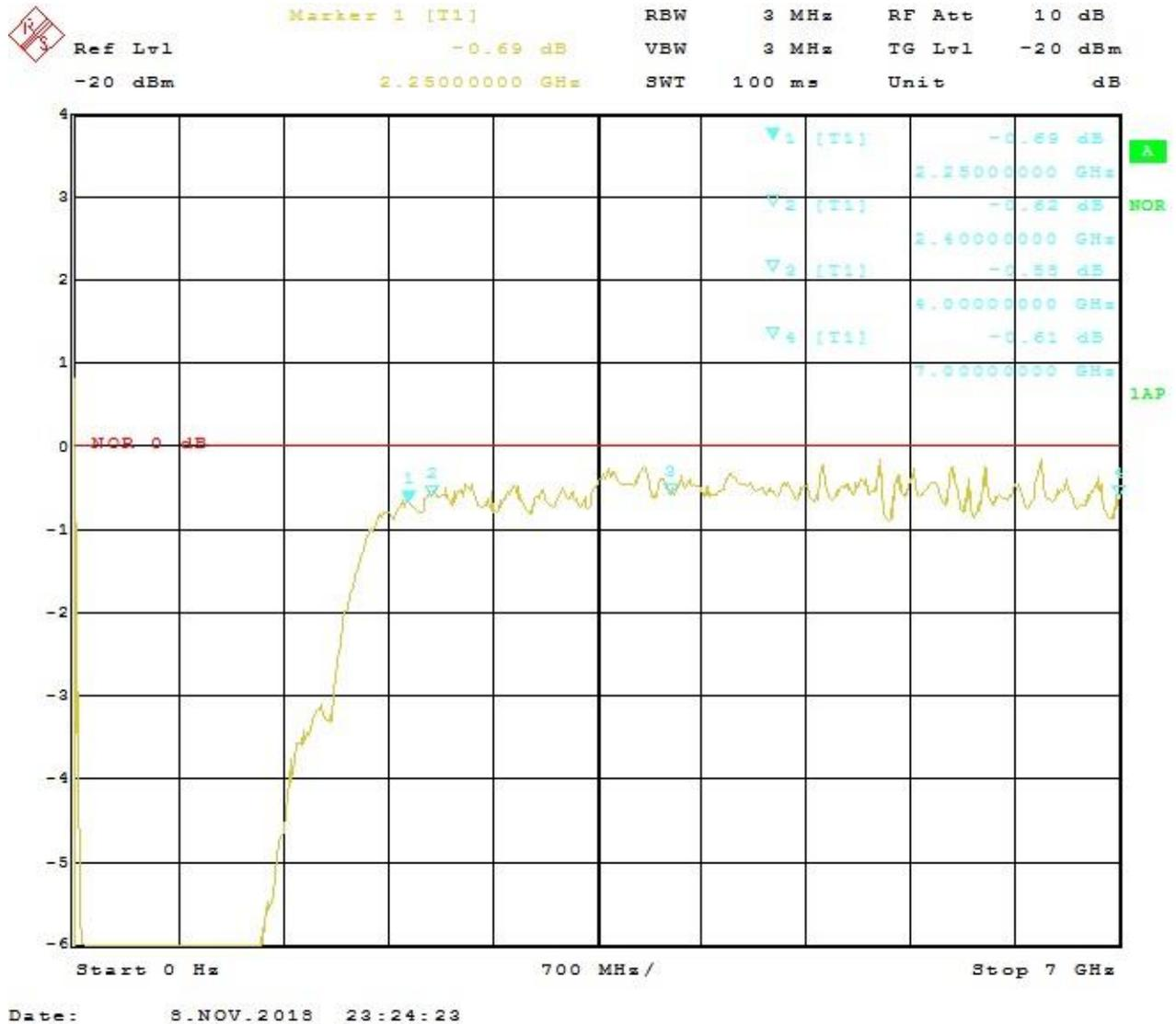
The insertion loss in the range ~2 GHz to 7 GHz is below 1dB. Here are some measurement points:
