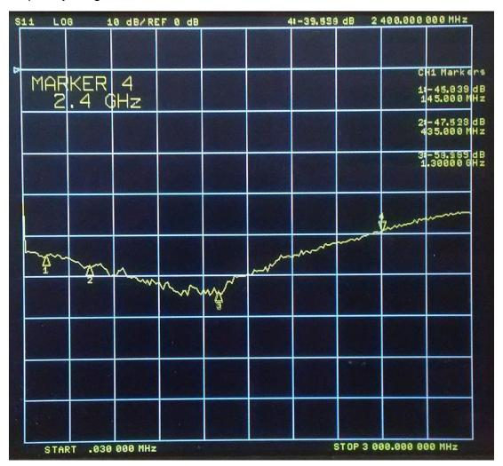
The return loss is 46dB at 145 MHz, 48dB at 435 MHz, 58dB at 1300 MHz and 40dB at 2400 Mhz. So it does serve well as a calibration load in my setup.
