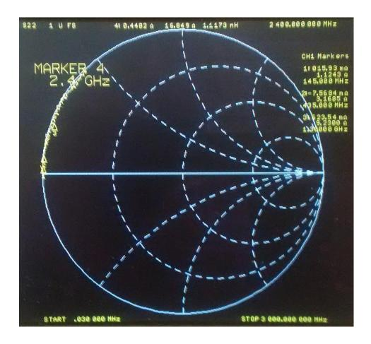
The open and the sort are only almost "ideal" at 145 MHz. With increasing frequency, the open and short are no more "ideal". Frankly I am not sure whether the measured values are good enough for a calibration unit and will have to look more into this.
