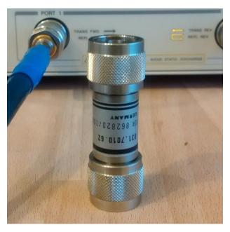
In addition, I acquired a 50 Ohm load with a N-plug, again not knowing any specifications on it. It is marked as Weinschel Model 1424-3.
