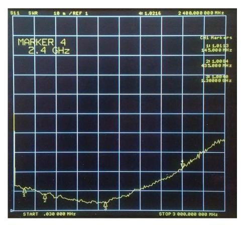
The SWR is 1.01 at 145 MHz, 1.01 at 435 MHz, 1.00dB at 1300 MHz and 1.02 at 2400 Mhz.
