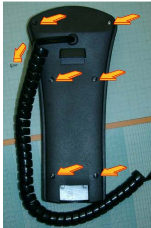
Hand controller rear side, the 6 screws like the one in the upper left corner have to be removed to open the hand-controller
