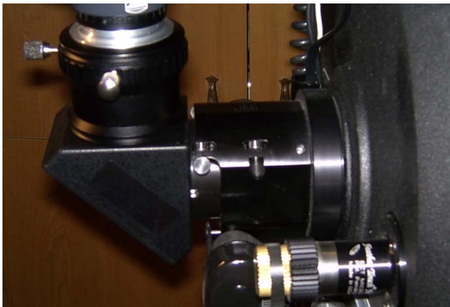
From left to right: Baader Planetarium Maxbright diagonal, NGF-S fully moved in, 3" Adapter ADPT3SCT
