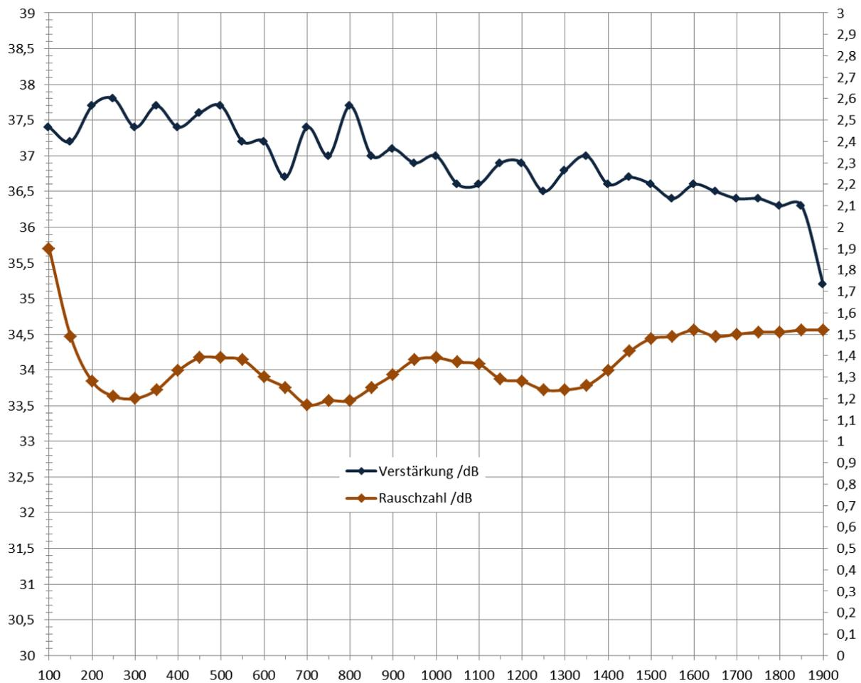
You can see that the gain (dark blue curve “Verstärkung” with the left scale) is quite constantly about 37dB in the range from 100 up to 1900 MHz and the noise figure (brown curve “Rauschzahl” with the right scale) at the same frequency range is about 1.2 to 1.5 dB.
