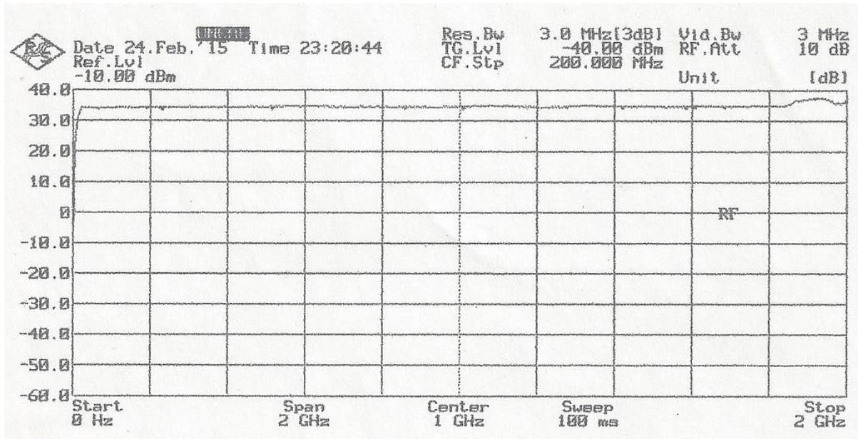
As can be seen the gain is very flat between about 30 and 2000 MHz with approximately 35 dB.
