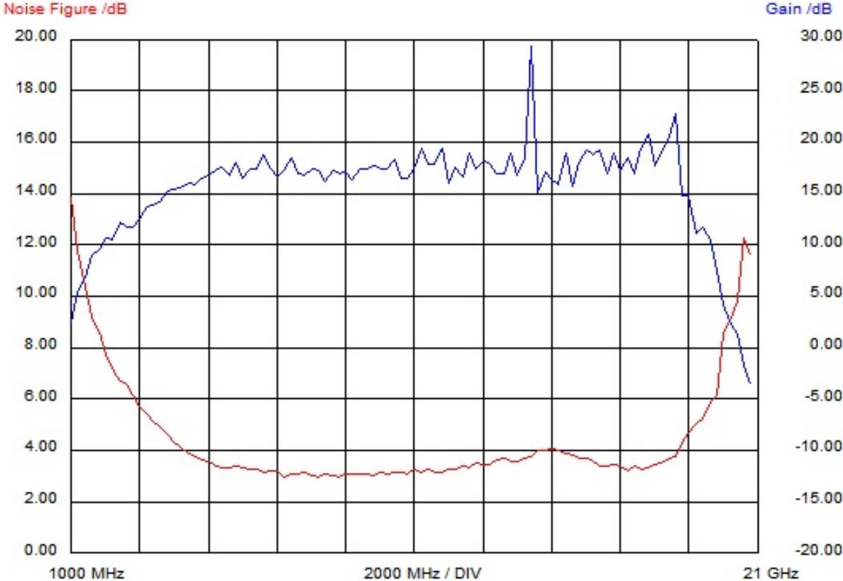
Between 5 and 18 GHz the gain is essentially the same (between 14 and 16dB besides the 2 peaks). The noise figure is lower (between 3.0 and 4.1 dB).
