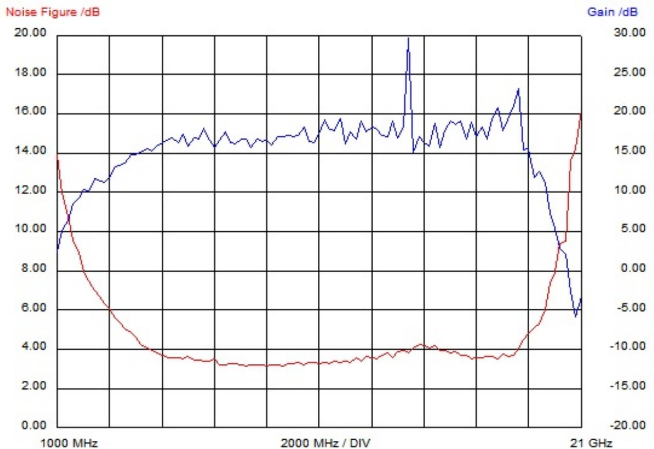
The results are almost identical to the 12V measurement. The noise figure is slightly higher.
