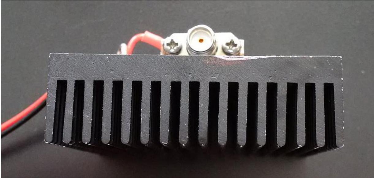
Next, I measured gain and noise figure versus frequency. The first measurement was done at the nominal supply voltage of 20V and a corresponding supply current of 110mA.
