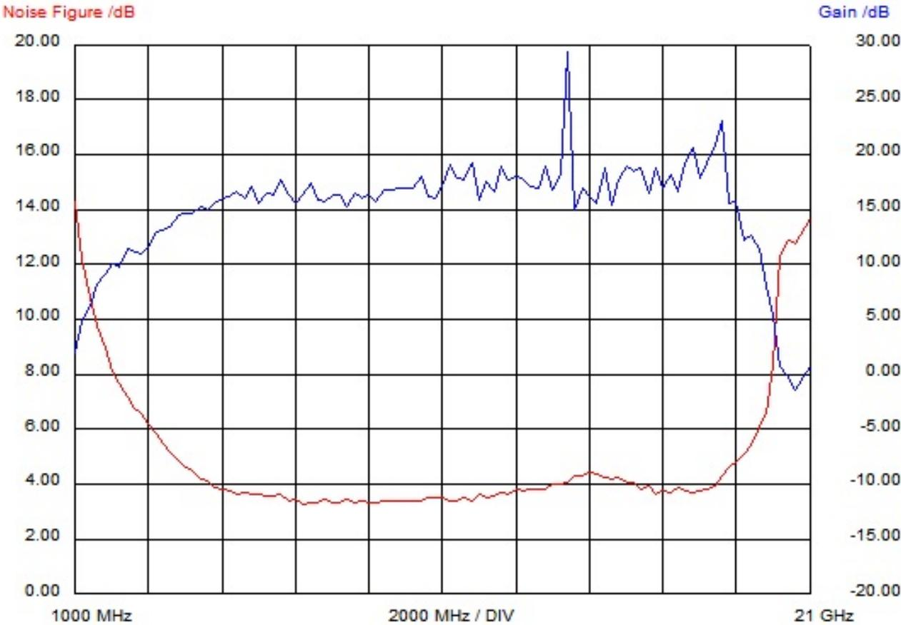
The frequency response is rather flat. In the frequency range 5 to 18 GHz the gain is between 14 and 16dB (besides 2 peaks) and the noise figure between 3.5 and 4.5dB.
