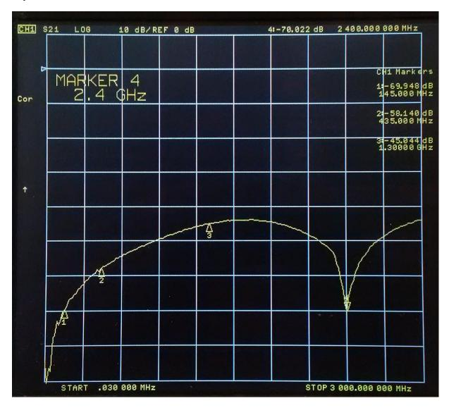
The resulting directivity is 25.6dB at 1.3GHz and 50.3dB at 2.4GHz respectively. This is significantly better than the specified value of >20dB. This coupler works especially well at the 13cm ham radio band.
