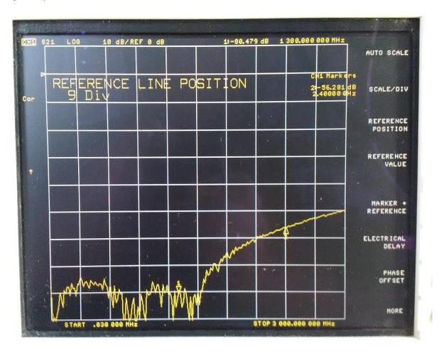
Finally, I measured the directivity, which is the ratio S31 to S32.
