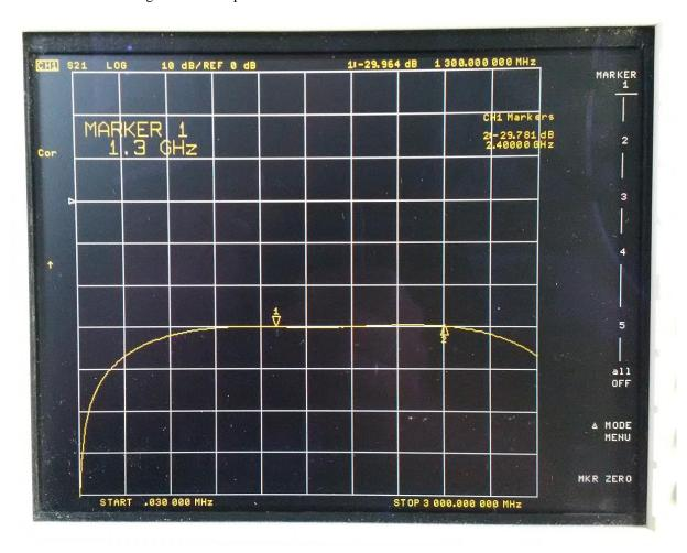
Next, I measured the isolation S23 from the output port to the measurement port. The input was again terminated with a high quality 50 Ohm load.
