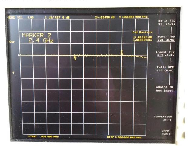
I have not tested the maximum power but the very low insertion loss indicates that there should be no problem. The insertion loss of 0.034dB means that using an input power of 200W less than 2W are dissipated in the coupler.
