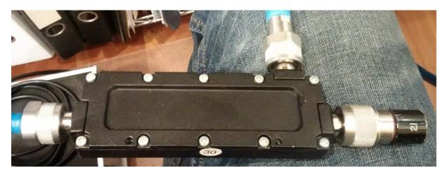
The isolation including the 30dB coupling factor was measured to be 58.6dB at 1.3 GHz and 63.9dB at 2.4 GHz respectively.
