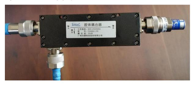
As can be seen in the next graph the coupling factor at 1.3 GHz was measured as 29.6dB and at 2.4 GHz as 29.8dB. This is amazing close to the specified value of 30dB for such a low-cost device.
