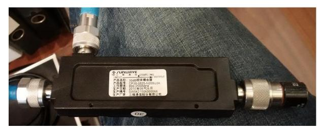
As can be seen in the next graph the coupling factor at 1.3 GHz was measured as 29.94dB and at 2.4 GHz as 30.19dB. This is amazing close to the specified value of 30dB for such a low-cost device.
