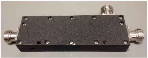
The N-connectors are really low quality. The outer thread is quite rough and I was afraid damaging the high-quality connectors of my measurement setup when screwing them onto the plugs of this directional coupler.
