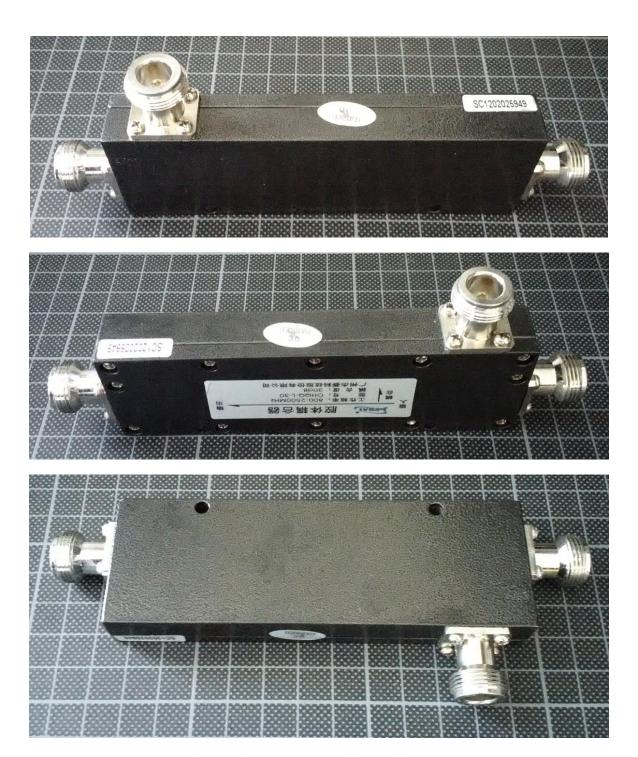
The N-connectors are not really high quality but should be ok if the unit is used in a permanent setup as I am planning for. The outer thread is reasonably precise so that the N-Connectors can be easily screwed on.
