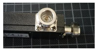
First, I measured the insertion loss S21 of the coupler from 30kHz to 3 GHz with the measurement port terminated with a high quality 50 Ohm load:
