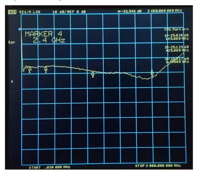
The directivity was measured to be 28.8dB at 1.3GHz and 32.5dB at 2.4GHz respectively. This is significantly better than the specified value of >20dB. This coupler works especially well at the 13cm ham radio band.
