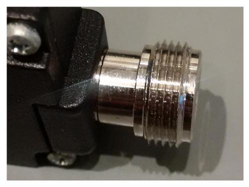
First, I measured the insertion loss S21 of the coupler from 30kHz to 3~GHz with the measurement port terminated with a 50~Ohm load:
