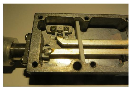
Please note that 50 Ohms termination resistor which is terminating one end of the measurement line. It is screwed to the aluminum encasing and I estimate that it should be capable of handling at least 20W RF power. With the coupling factor of 20dB that would be equivalent to an input power of the directional coupler of 2kW.
