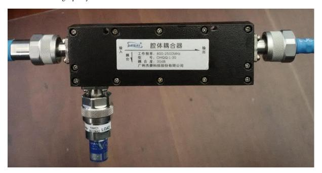
As can be seen in the next graph the insertion loss at  $1.3 \, \text{GHz}$  was measured as  $0.012 \, \text{dB}$  and at  $2.4 \, \text{GHz}$  as  $0.034 \, \text{dB}$ . This is well in the spec of better than  $0.05 \, \text{dB}$ .
