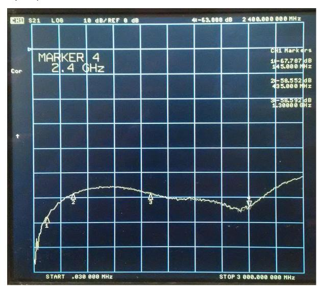
Finally, I measured the directivity, which is the ratio S31 to S32.
