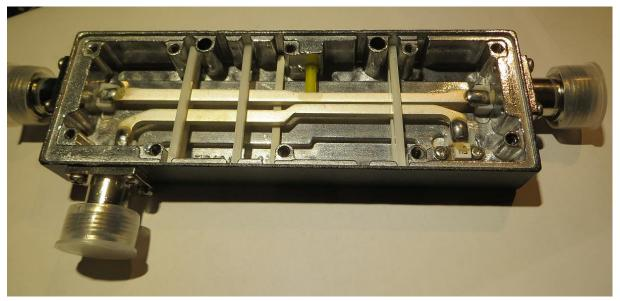
Please note that yellow plastic screw which can be moved from outside. This screw is pushing against the upper transmission line (bar) and thus the distance to the second line can be adjusted. Thus the coupling factor can be tuned in production. After alignment a sticker like QC or similar is glued over the screw to hide / protect it.
