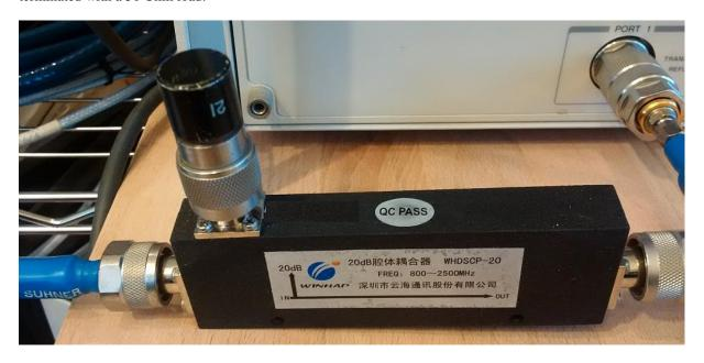
As can be seen in the next graph the insertion loss at 1.3GHz was measured as 0.087dB and at 2.4 GHz as 0.156dB. These values are slightly worse than the specified values of better than 0.05dB.
