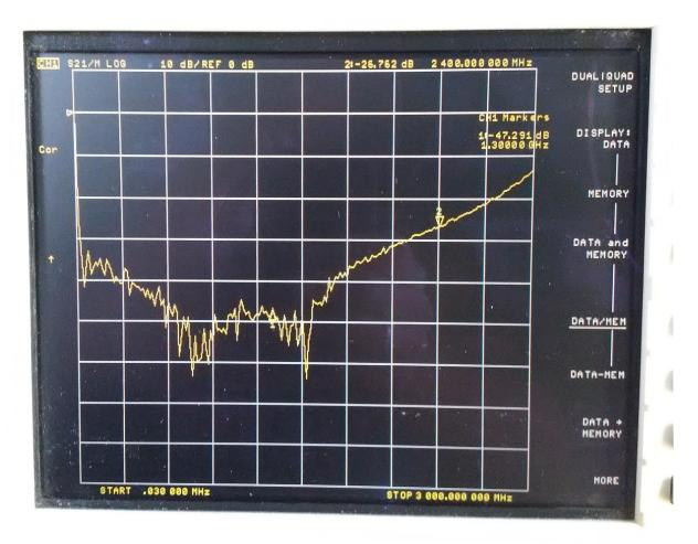
The directivity was measured to be 47.3dB at 1.3 GHz and 26.8dB at 2.4 GHz respectively. This is significantly better than the specified value of >20dB. This coupler works especially well at the 23cm ham radio band.
