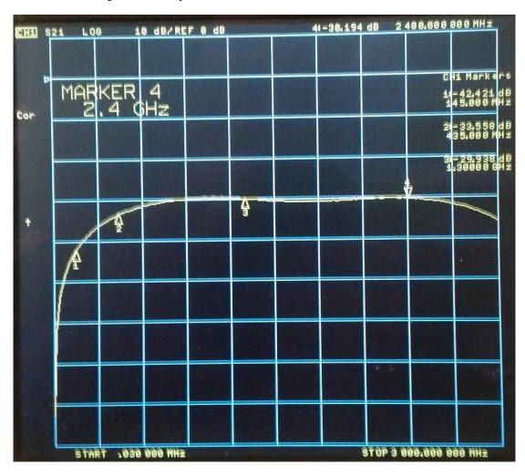
Next, I measured the isolation S23 from the output port to the measurement port. The input was again terminated with a 50 Ohm load.
