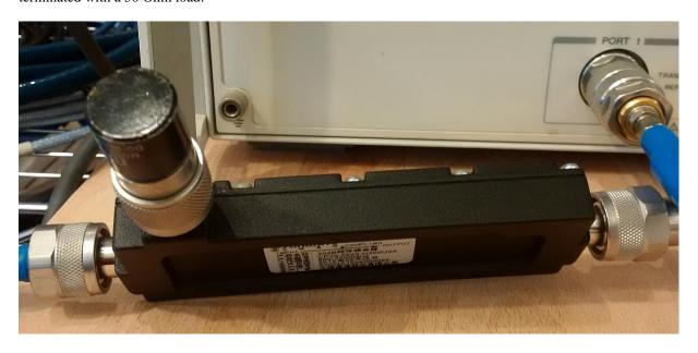
As can be seen in the next graph the insertion loss at 1.3GHz was measured as 0.08dB and at 2.4 GHz as 0.12dB. This is slightly higher than the spec of better than 0.05dB.
