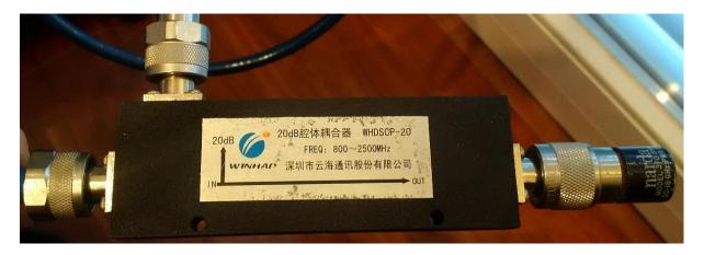
As can be seen in the next graph the coupling factor at 1.3 GHz was measured as 19.55dB and at 2.4 GHz as 19.75dB. This is amazing close to the specified value of 20dB for such a low-cost device.
