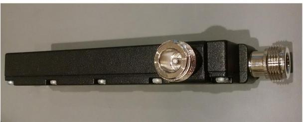
The N-connectors are not really high quality but should be ok if the unit is used in a permanent setup. The outer thread is reasonably precise so that the N-Connectors can be easily screwed on.
