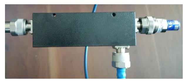
The isolation including the 30dB coupling factor was measured to be 80.5dB at 1.3 GHz and 56.3dB at 2.4 GHz respectively.
