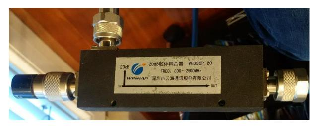
As can be seen on the next plot the isolation including the 20dB coupling factor was measured to be only 45dB at 1.3 GHz but amazing high 70dB at 2.4 GHz. Exactly at 2.4 GHz this coupler shows a strong resonance with respect to its isolation.
