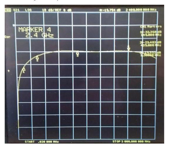
Next, I measured the isolation S23 from the output port to the measurement port. The input was again terminated with a 50 Ohm load.
