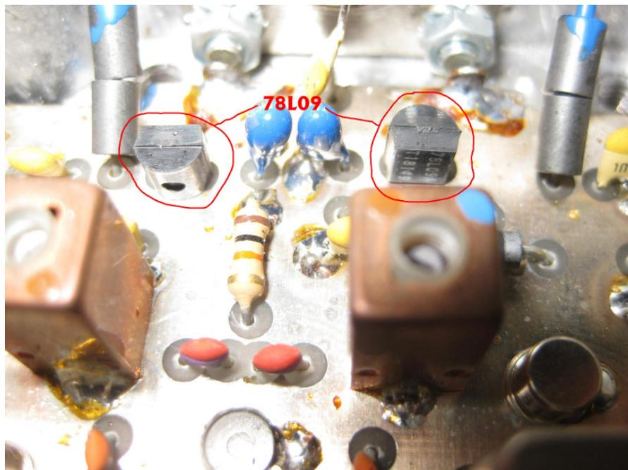
Each channel of the downconverter has its own voltage regulator. I recognized the two ferrit beads per channel that are threadlocked to the power input wires.
