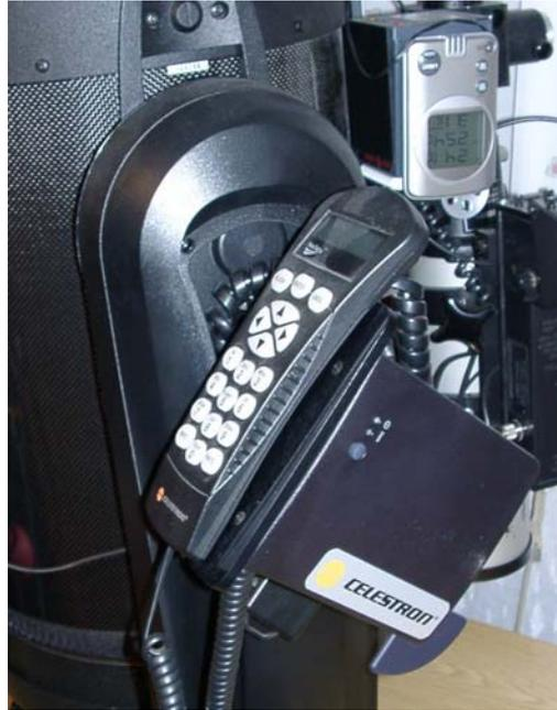
Frank Dilatush found a solution in the Astroshop "S&S Optika" in Colorado. It is a holder for the hand-controller which can be attached to the fork arm without altering it in any way. The bracket is clamped in a clever way in the cavity where the hand-controller is usually placed. The hand-controller is placed on the bracket and is now turned 90° versus its original position. The vertical angle of the bracket can be freely adjusted depending on the taste of the user.
