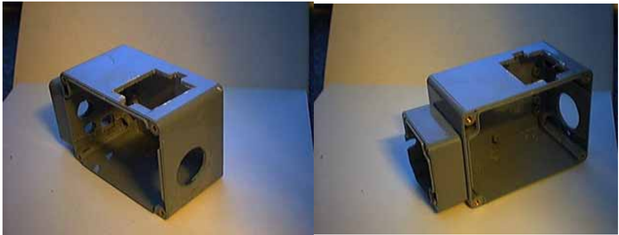
Image 1 PVC boxes with the necessary holes for the cooling block, the 1.25" adapter and cable connectors
