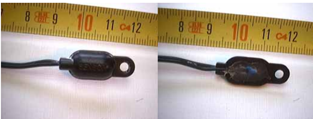
Image 4 Outdoor temperature sensor with scale in cm's. LEFT : Front view. RIGHT: Back view
