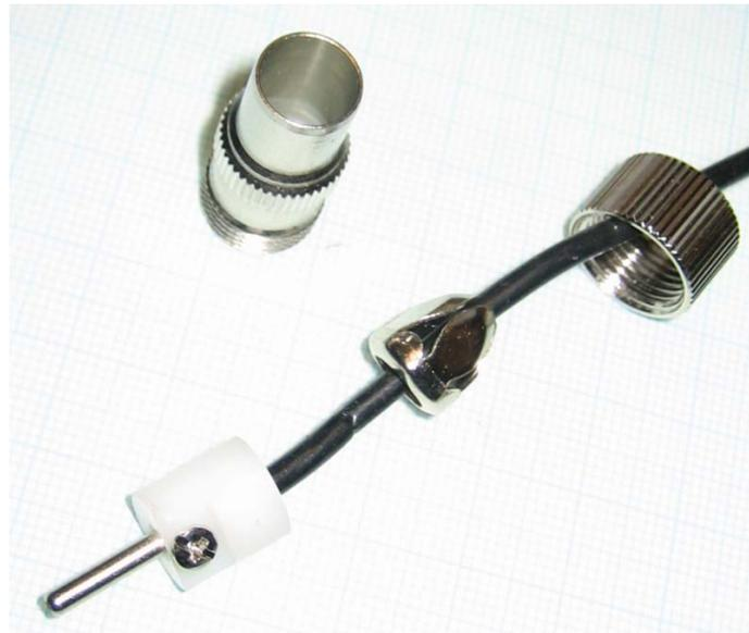
Hm, this is not really a coaxial cable .. it is a simple wire only attached to the center pin of the coaxial connector ... and the other side of the wire is attached to a piece of PCB without any sense ... cut the whole thing off and the wire will still act as the antenna ....
