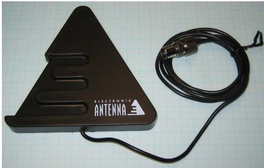
Looks interesting, doesn't it ? The black coaxial cable is approximately 2m long and a metal shielded coaxial connector as normally used for TV systems is attached to it. Here are some more pictures of the front and back of the neat little antenna.
