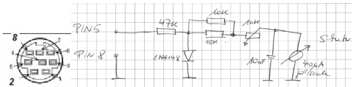
The general definition of the S-meter scale is a function of frequency. At frequencies below 30 MHz the reference value S9 corresponds to an input power level of -73 dBm. At frequencies above 30 MHz S9 corresponds to an input power level of -93 dBm. Each step to a lower level equals a reduction of the input power of 6dB which is 1/4 of the previous power level. You can find the levels in the table below.
