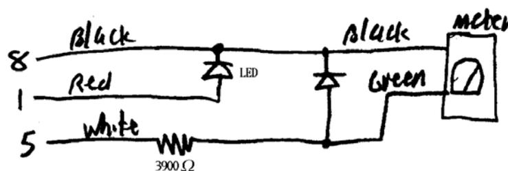
I checked my drawers for surplus electronics parts and found a nice large moving-coil instrument with a 40um full scale reading. It even features a mirror behind part of the scale which makes the reading of the needle quite easy. I developed the small circuit which you find in the sketch below to attach it to PIN5 (RSSI output) and PIN8 (ground) of the ACC port of the AR8600.
