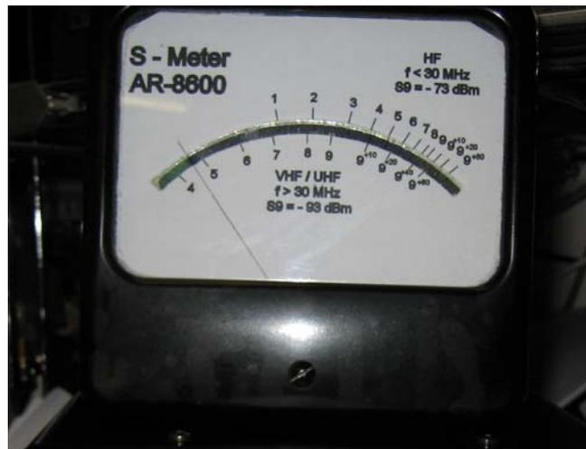
By the way: my S-meter shows consistent results using an un-modulated carrier and in conjunction with the different demodulator settings except for using WFM. The reading is constant (as it should be) using all other demodulator settings. However in WFM mode, which I use only to receive FM broadcast stations around 100 MHz, the reading is quite different. I am curious to get feedback from other users whether they made the same observations.
