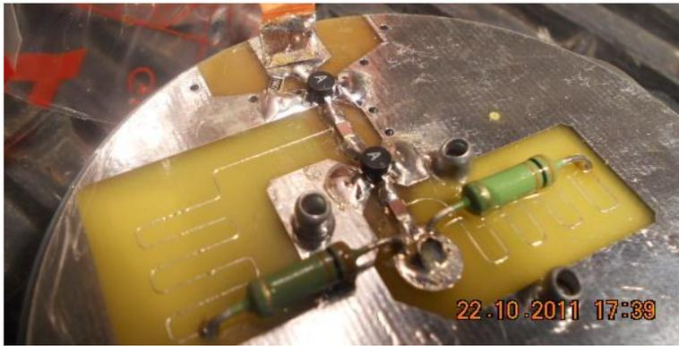
The MSA-1105 MMIC is a high dynamic range 50 Ohm or 75 Ohm gain block with a 3dB bandwidth of 50 MHz to 1.3 GHz. The 1dB compression point at 500 MHz is P1dB=17.5 dBm. The typical noise figure at 500 MHz is 3.6 dB. The package is a “05” surface mount
