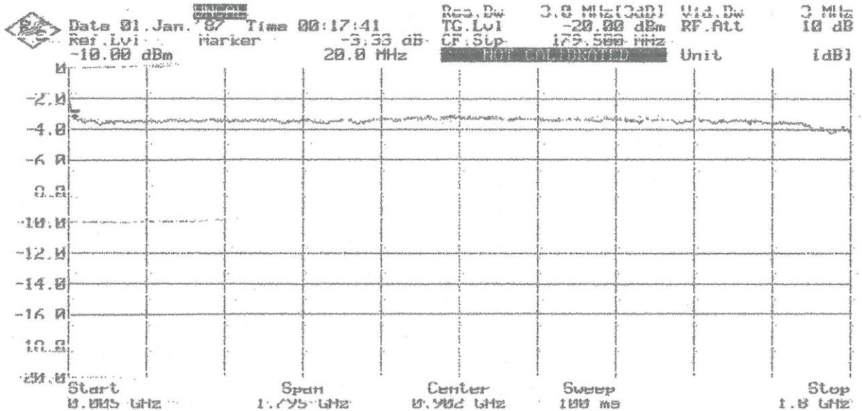
We can see a very nice flat frequency response down to about 20 MHz if the second port is properly terminated. The insertion loss is about 0.5dB over a wide range at increases to 1dB at 1750 MHz.
