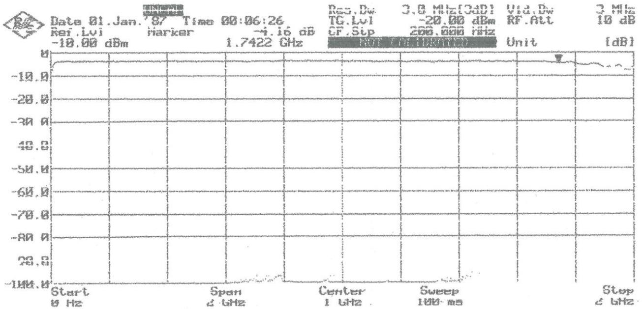
The result is very similar to the measurement before. The splitter shows a nice symmetrical behavior.
