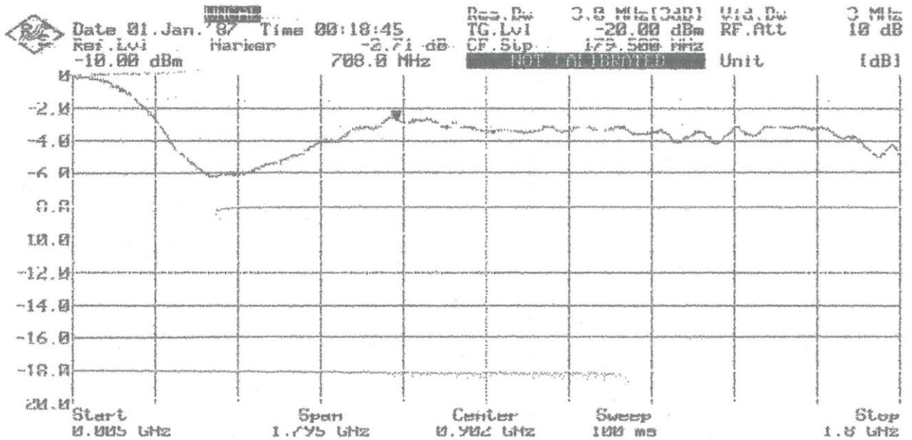
Finally, I verified the symmetrical behavior of the power splitter by repeating the measurement from the input port to output port #2 (without DC path).
