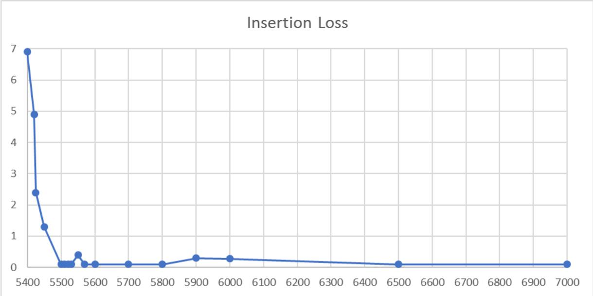
Next I repeated the same measurements, using again port “1 S-C-X” as input port but this time port “3 S-X” as the output port. Port “2 C” was terminated with 50 Ohms.
