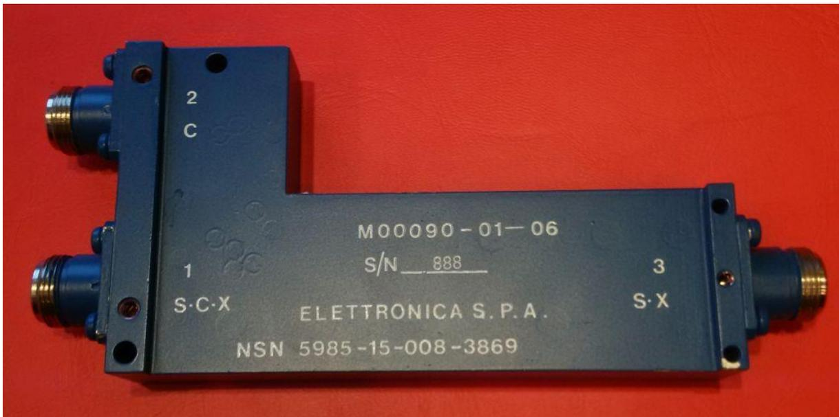
The diplexer has 3 ports with the names „1 S-C-X“, „2 C“ and „3 S-X“. The connectors used are all N-type.
