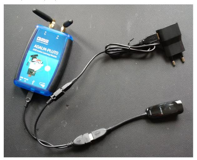
ADALM Pluto (upper left) connected by a USB OTG adapter cable (lower left) to a USB-Ethernet adapter (lower right). By the additional port of the Y-cable the USB-Ethernet adapter and the Pluto are powered by a 5V power supply.
