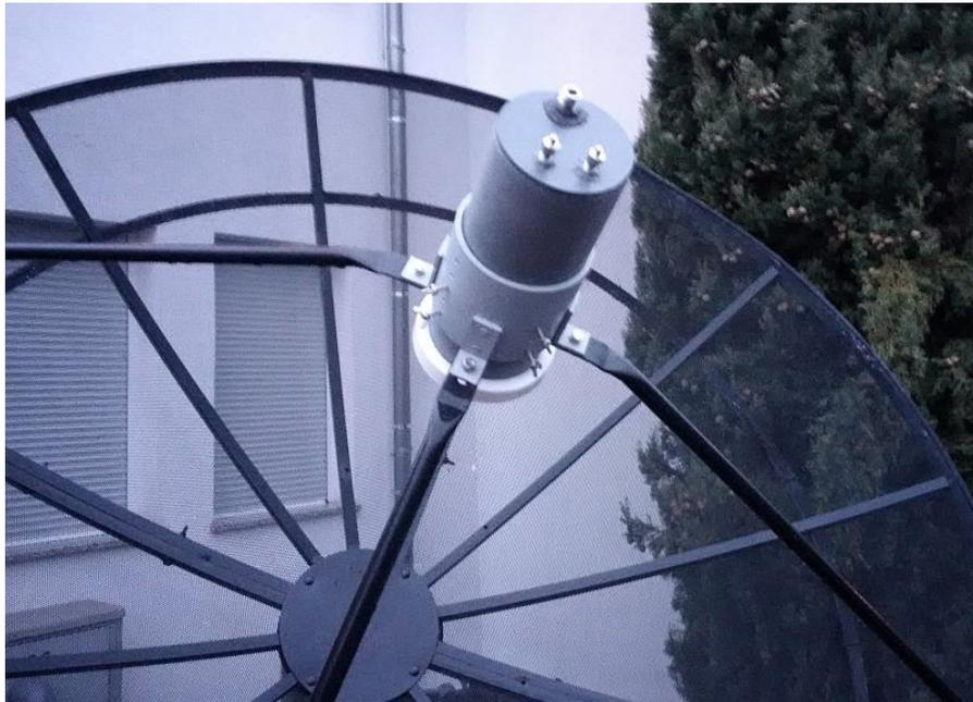
In order to fit my POTY feed in the same plastic tube as the previous feed I had to reduce the diameter of the reflector slightly. All parts of the feed are made from brass and are soldered. Here are some pictures:
