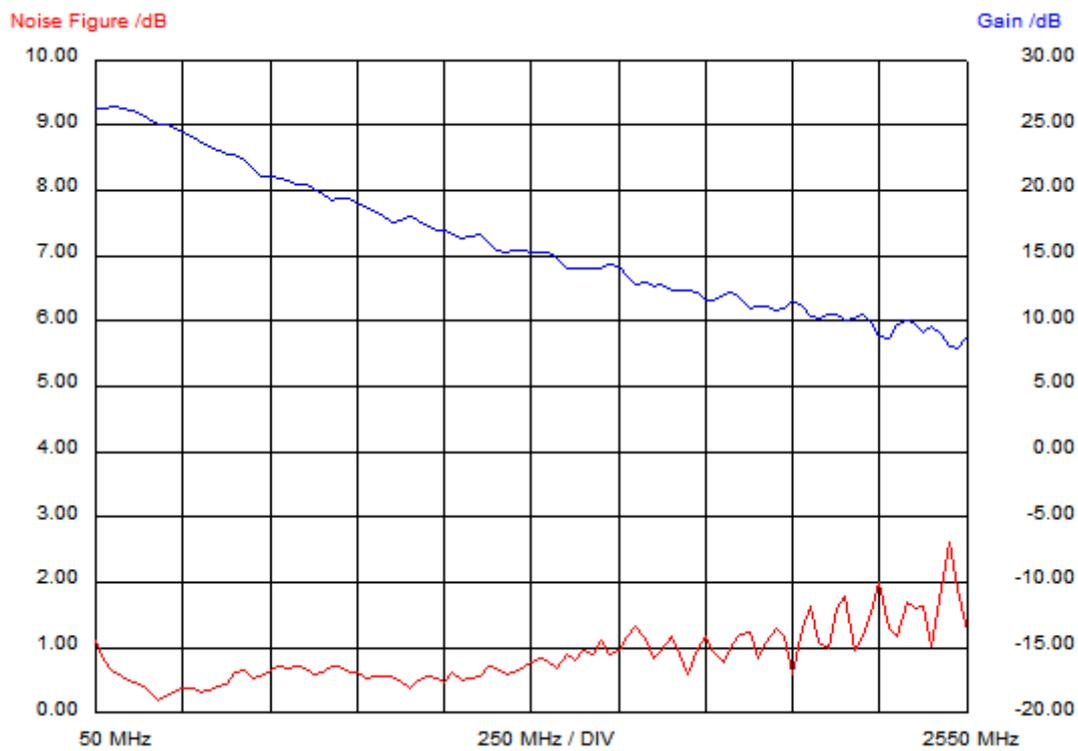
As can be seen the LNA features a maximum gain of about 26 dB below 150 MHz. The gain drops to 23 dB at 400 MHz and 20 dB at 700 MHz. At 1300 MHz the gain is down to about 13 dB and at 2400 MHz it is below 10 dB. A minimum noise figure of 0.2 dB is achieved at 225 MHz. The noise figure at 145 MHz is below 0.5 dB and at 435 MHz below 0.6 dB. At 1300 MHz the noise figure is still below 0.8dB.
