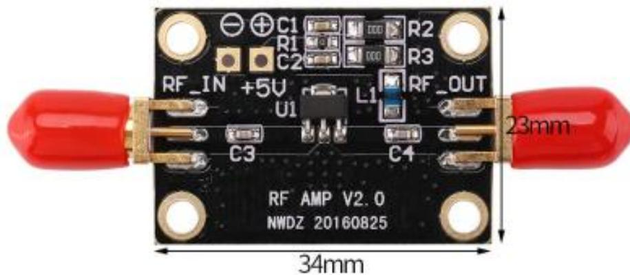
Next, I measured the gain and noise figure in the frequency range 50 MHz to 2550 MHz.
