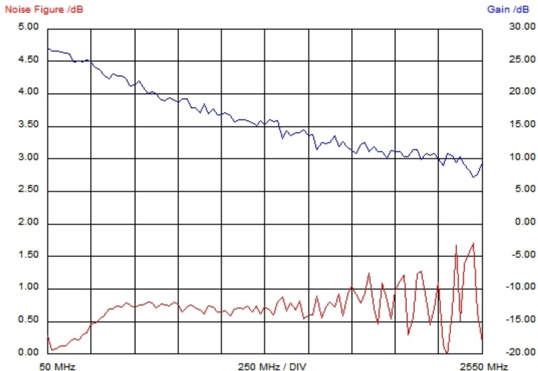
Even though this amplifier is not really useful up to 4 GHz it provides excellent performance in the VHF/UHF range and can certainly be used successfully for terrestrial operation in the 23cm band. Even in 13cm band it can be used with some compromised (lower gain and higher noise figure)
