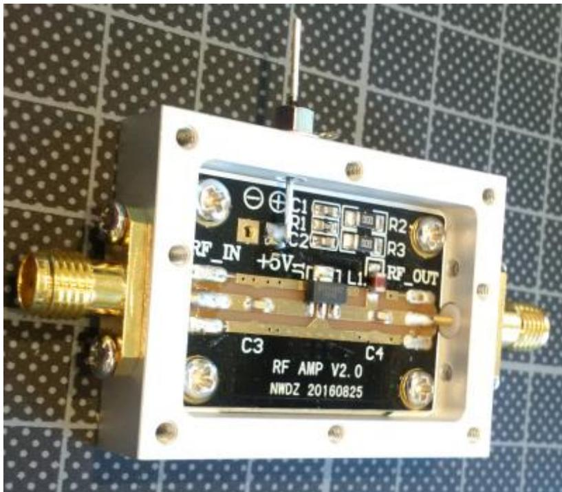
The amplifier is based on SPF5189Z, a GaAs MMIC from Quorvo. The datasheet values of this MMIC correspond well with the specified value of the amplifier. There is no voltage regulator inside, thus the supply voltage should be  $5V \pm 250mV$ . The measured current consumption is 90mA @5V. The output power at 1dB compression point is about 22-23dBm.
