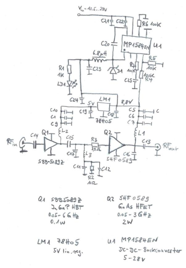
The schematic and also the layout of the PCB are almost identical to the 1W version using an SHF0289 MMIC in the second stage (see separate report).
