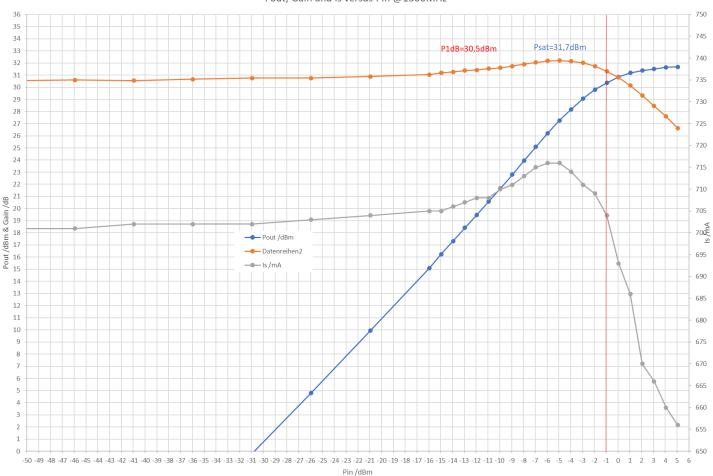
Pout, Gain and Is versus Pin @1300MHz
