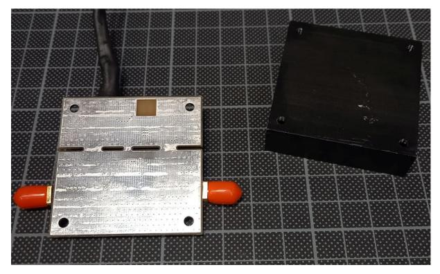
Therefore, I added 2 M3 screws close to the second MMIC (see later photograph) and mounted the PCB on the heatsink with some thermal grease (Arctic 5). In addition, I put a metal shielding around the PCB and replaced the original SMA sockets with large SMA flange sockets. This makes the whole setup mechanically and electrically much more robust.
