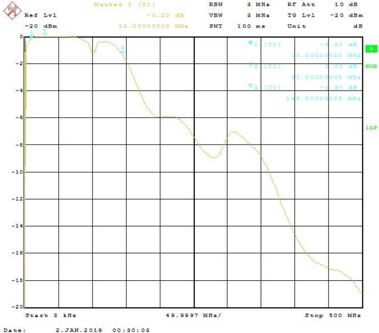
The insertion loss at 10 MHz is 0.2dB and even at 145 MHz is still below 2dB. The attenuation at 500 MHz is almost 20dB.
