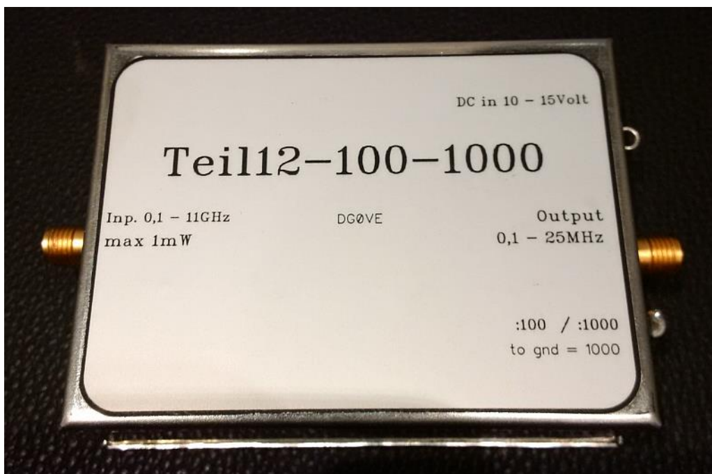
The prescaler is housed in a tin-plated cabinet with high quality SMA connectors
