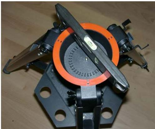
Next you need to attach a marking to the fixed and the movable part of the mount. I used a self adhesive barcode label as can be found on the German postal labels. I made it weather proof by covering it by a transparent foil on top of it.
