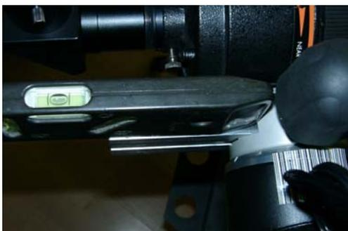
In subsequent alignments you can now easily perform the orthogonal alignment within seconds without the need to use a level.
