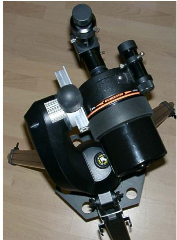
If you dislike the small tray in the tripod if the GT telescope you easily enlarge it by adding an additional sheet underneath. I cut holes into the black plastic sheet and can now securely store my 1 1/4" eyepieces while not in use.
