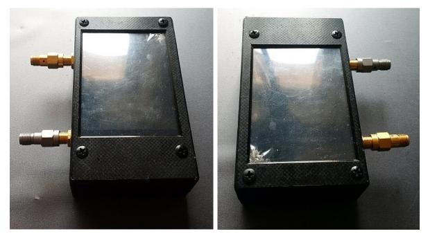
In the pictures you can also see the "Connector Savers" which are SMAm-SMAf adapters which protect the original SMA jacks of the NanoVNA V2. Once they are worn out, they can be simply replaced.
