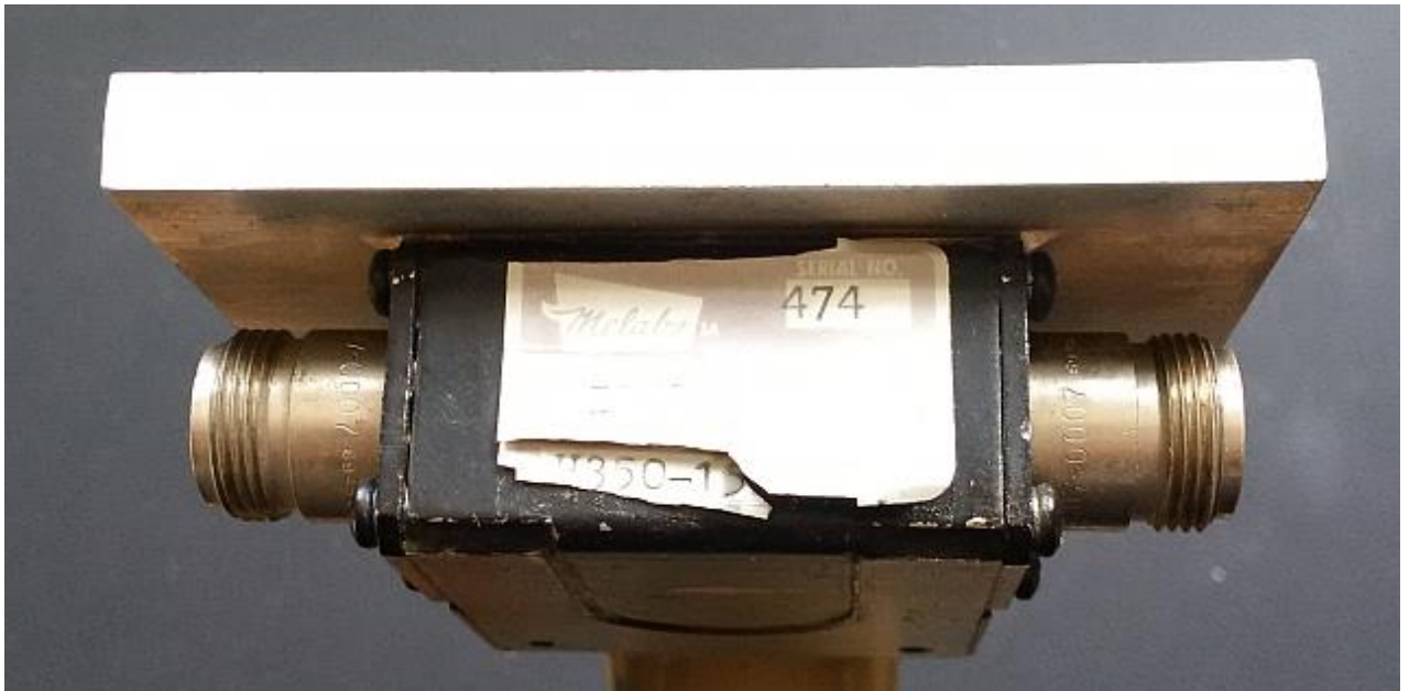
The input and output ports are equipped with 50 Ohms N-jacks.
