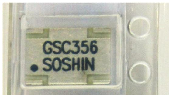
These couplers are perfect for the 2.4 GHz uplink frequency band of QO-100 and they can handle up 100 Watt continuous output power as they are designed for power amplifiers in base stations.
