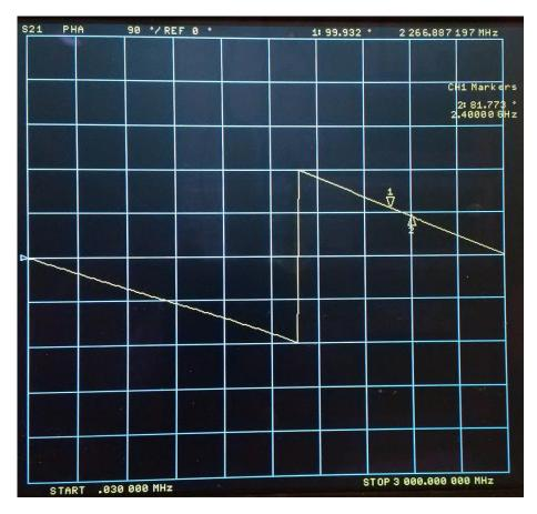
S21 phase at 2267 MHz is 99.93 degree, at 2400 MHz it is 81.77 degree.
