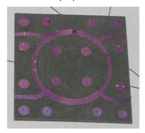
I cleaned the Teflon PCB and silver plated it. Then I mounted it on a surplus brass plate (which is gold plated which makes it look like (5)) in order to be able to test it.
