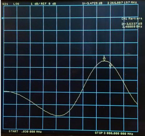
S21 log mag at 2267 MHz is -3.47dB. S21 log mag at 2400 MHz is -3.64dB.
