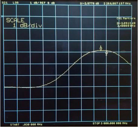
S21 log mag at 2267 MHz is -2.88dB. S21 log mag at 2400 MHz is -2.89dB.
