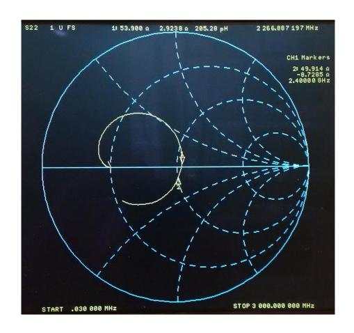
Finally, I measured the characteristic from port 2 to port 1:
