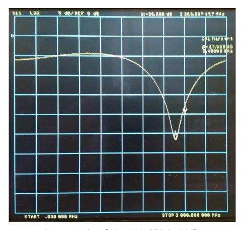
Input return loss S11 at 2267 MHz is -26dB. At 2400MHz the return loss S11 is only -18dB.
