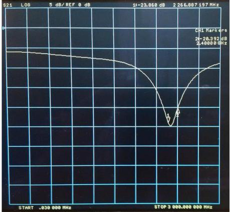
S21 log mag at 2267 MHz is -23.9dB. S21 log mag at 2400 MHz is -20.4dB.
