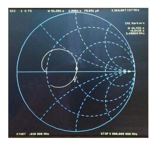
This is the summary of the parameters of the hybrid coupler measured at 2267 MHz:
