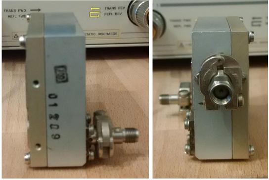
The circulator is in a solid metal case and has 2 unknown connectors. I think it is a SIEMENS type but I am not sure. They are adapted to SMA.
